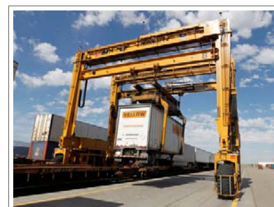
Al Hartmann | The Salt Lake Tribune Huge moving crane off-loads semi truck trailers with goods from rail cars at Union Pacific's intermodal shipping container hub at 5600 West and 10th South on July 12 2012. The huge hub offloads containers from trains and trucks pickup the loads for delivery throughout the intermountain west.
