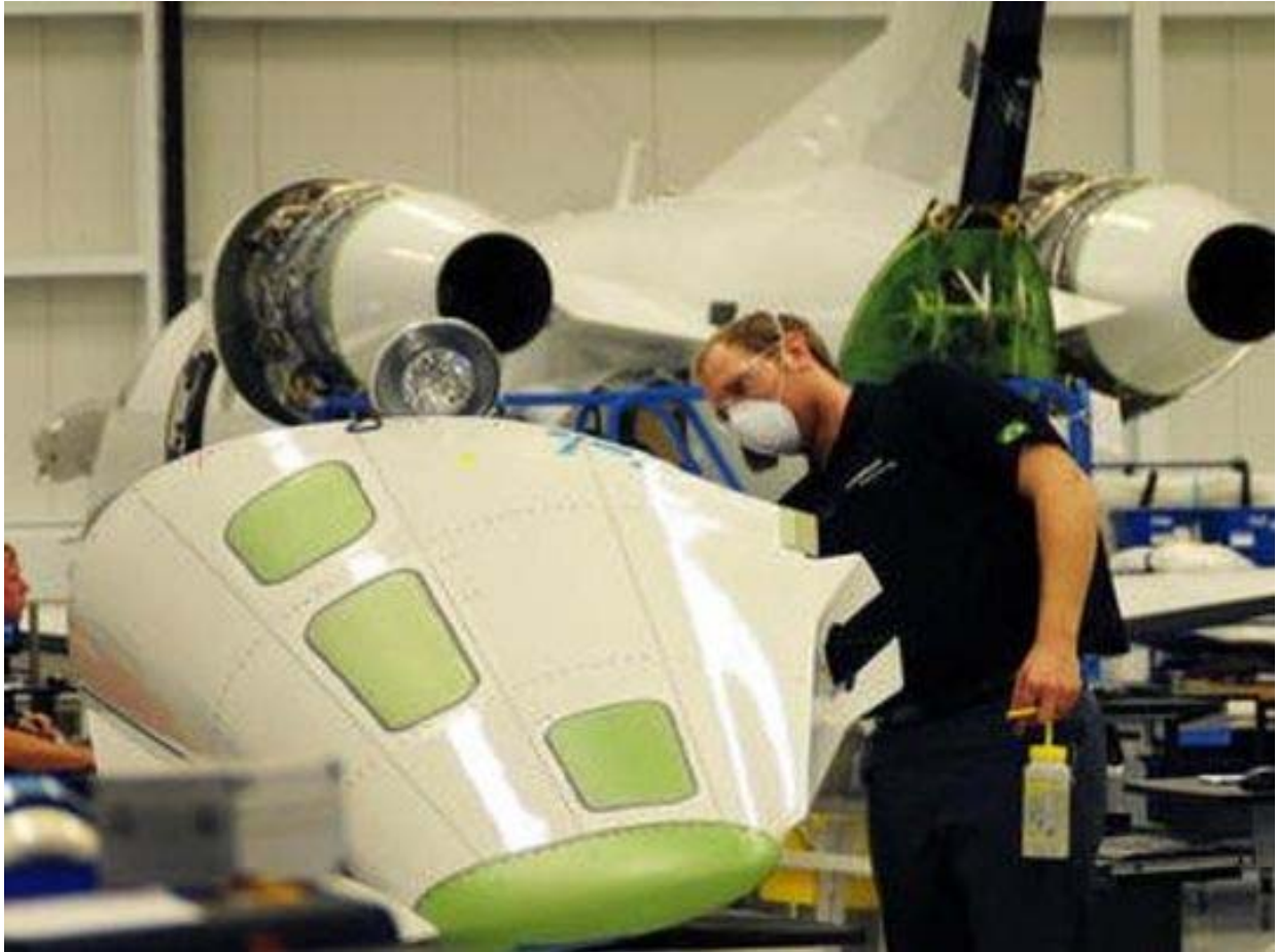
An Embraer assembly technician at work on the tail cone of a Phenom 300 in the Phenom Final Assembly Facility at the Embraer Executive Jets in Melbourne. (Photo: TIM SHORTT/FLORIDA TODAY)
