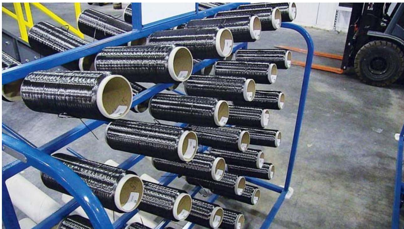
*Carbon fiber spools staged for packaging. Solvay makes the fiber in Greenville, S.C.*
